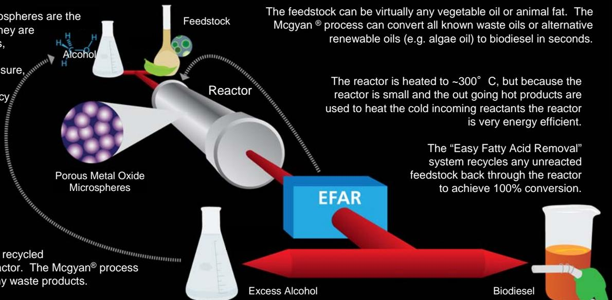
The feedstock can be virtually any vegetable oil or animal fat. The Mcgyan<sup>®</sup> process can convert all known waste oils or alternative renewable oils (e.g. algae oil) to biodiesel in seconds.
